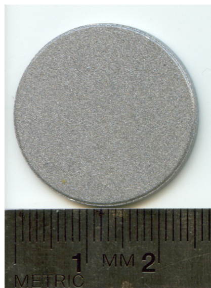
Fig. 3. Porous SS430 metal substrate.
